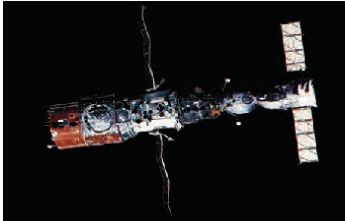
Salyut 6 Soviet Orbital space station with Soyuz spacecraft docked (right). Image source: http://www.spacefacts.de/graph/photo/photos2/soyuz-t-4_salyut.jpg
